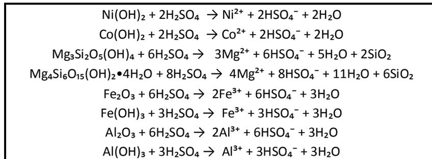
The hot slurry is sequentially depressurised and the steam released is recycled to pre-heat the incoming feed. The depressurised slurry is neutralized with limestone to precipitate the dissolved iron and aluminium. In this model no primary neutralization is done out with saprolite, as has been included in some flowsheets to reduce the acid consumption per unit of nickel dissolved, because this exercise looks at the two laterite types separately.
