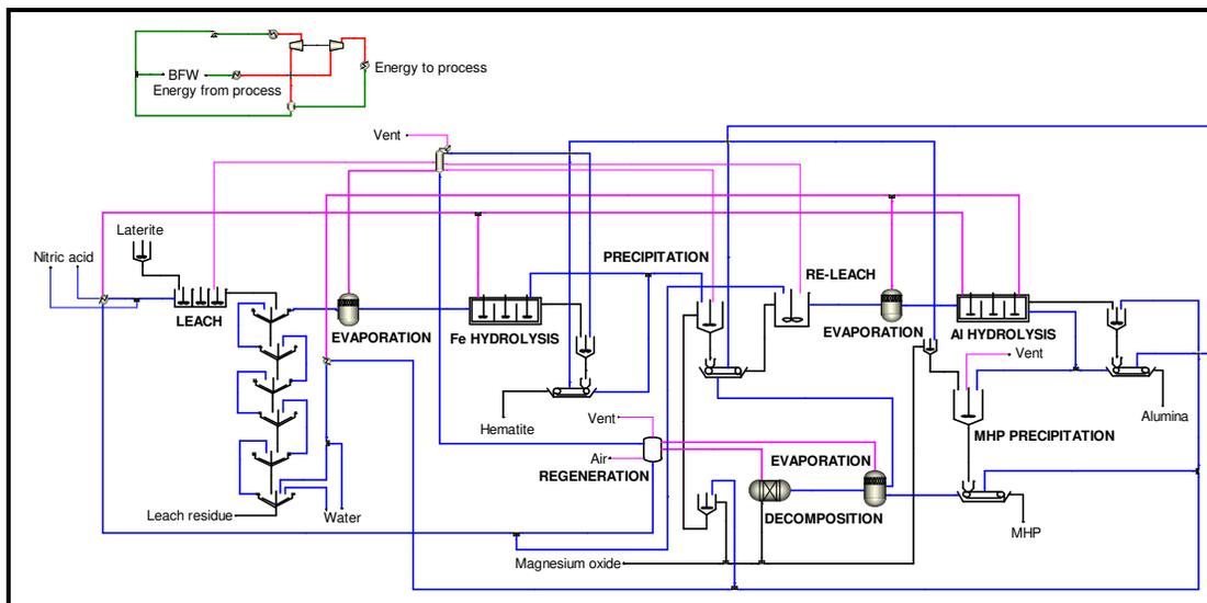
Figure 3 – Nitrate circuit
