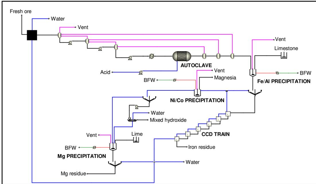
Figure 1 – Sulphate circuit
